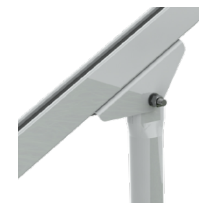
VGPCF10E series pile and sloped supporting frame top connected with diagonal beam bottom by hinger and fastener
